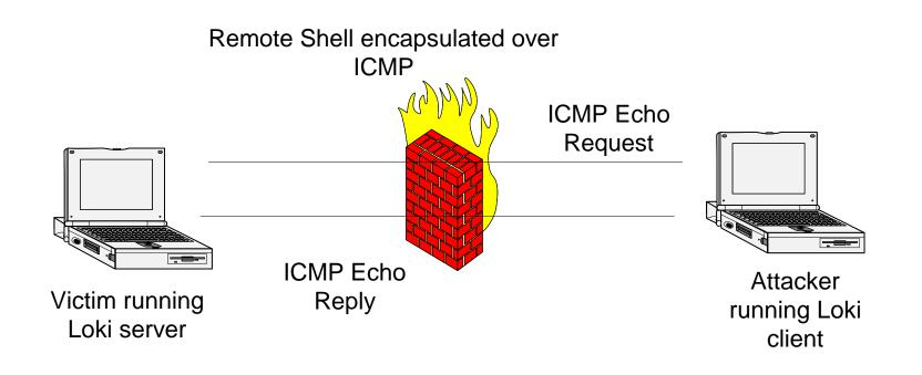
• Commands are encapsulated in ICMP Echo Requests/Replies are delivered in ICMP Echo Reply
