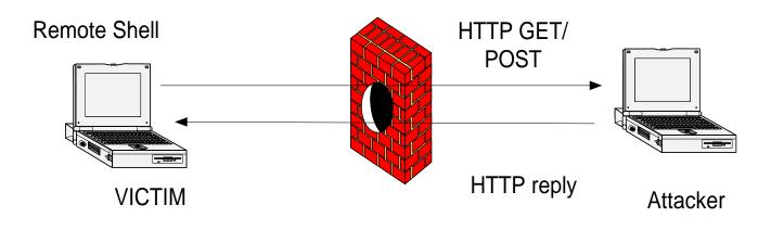
Shell commands / results are encapsulated in HTTP (POST/GET or replies) Firewall « sees » only outgoing regular HTTP traffic Difficult to detect....
