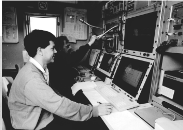
recording truck in exploration survey
